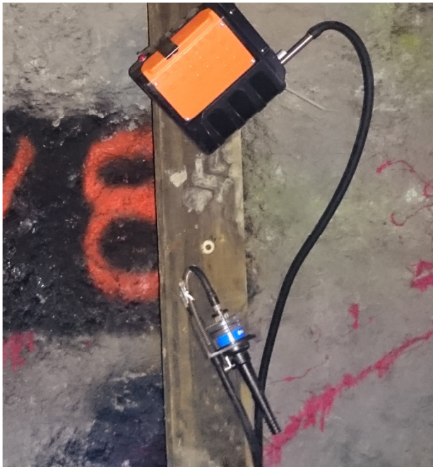
Figure 3. Real time DPM measurement instrument (Airtec).
